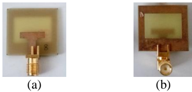
Figure 4. Fabricated transducer (a) top conducting layer (b) ground plane
